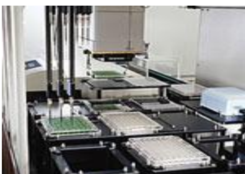
Figure 1: Biomek® FXp Laboratory Automation Workstation: Dual Arm System with Multichannel Pipettor and Span-8 Pipettor (Beckman, PN: A31844)
